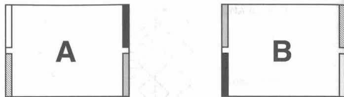
FIGURE 8.11: The two tile types for DNA self-assembly. The shaded edges denote sticky ends that bind to complementary sticky ends on the opposite tile with the same shading.
